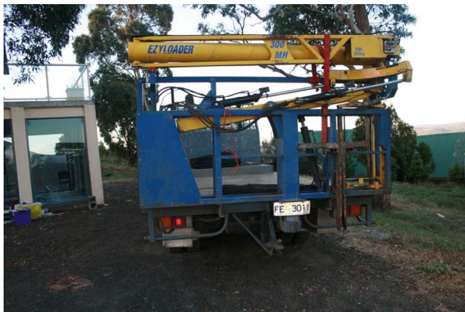
This truck is fitted with a purpose-built loader.
